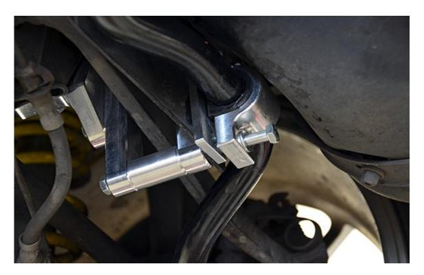
**Step 11** – Tighten the M8 and M10 subframe brace hardware that you left loose in Step 4 and Step 5. You will need to tighten the top M10 bolts and nuts first, then the bottom ones.
