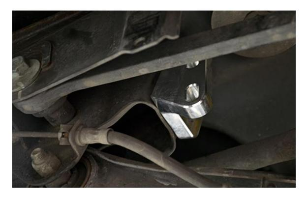
**Step 5** – Slip the subframe brace u-brackets over the tie rod and position the appropriately in the subframe. Using the M8x35 bolts and M8 washers, secure them to the left and right subframe brace brackets. **Do not tighten the hardware completely, so that you can adjust the alignment of the brackets during installation.**
