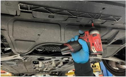
**Step 3** Using a 16mm wrench, remove the hardware from the axle guard, and set it aside.
