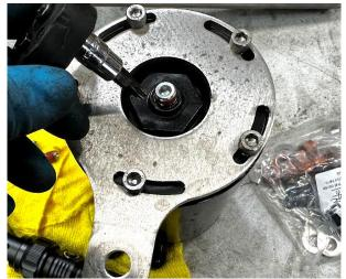
**Step 16** Using an 11mm wrench, install the 90° NPT fitting into the bottom of the catch can.
