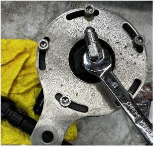
**Step 17** Install the braided line onto the 90° NPT fitting.
