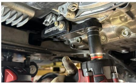
**Step 12**Using an 18mm socket, remove the steering rack hardware.
