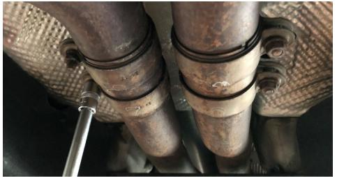
**Step 4** Using exhaust hanger pliers, separate the front hanger from the bushing.
