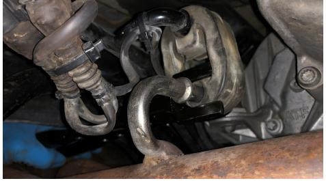
**Step 6** Using a 13mm socket, remove the rear exhaust hanger hardware.
