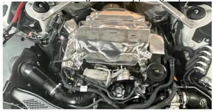
**Step 3**Unbutton the heat jacket from the fuel lines.
