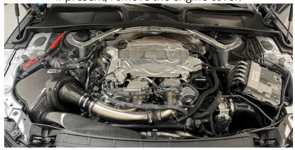
**Step 3**Unclip the ECU from the bracket.
