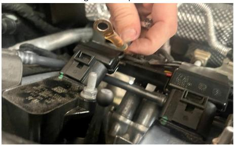
**Step 5**Carefully disconnect the coil harness plugs from the coils.
