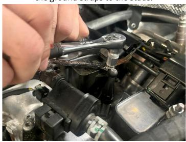
**Step 4**Remove the ground straps from the studs.
