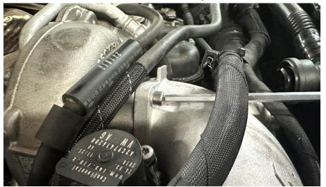
**Step 19** Attach the lower PCV hose to the SüperDüper turbo inlet.
