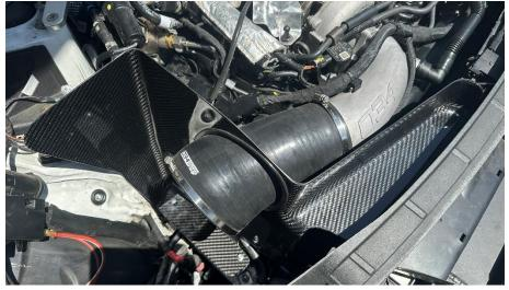
**Step 25** Attach the hose coupler to the intake hose.
