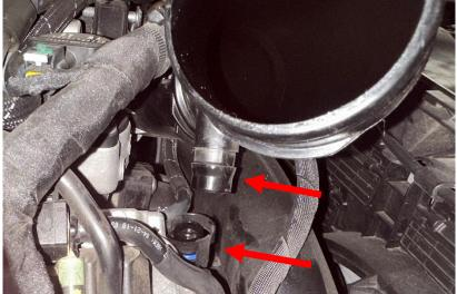
**Step 13** Extract the factory turbo inlet pipe (Don't mind the intake components still installed in this picture).
