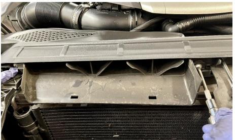
**Step 5** Remove the fresh-air duct.
