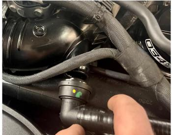
**Step 11** Using a T30 Torx, remove the hardware to release the factory turbo inlet from the turbo. The bolt on the underside can be
