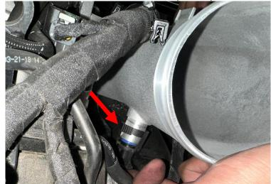
**Step 17** Slide the SüperDüper turbo inlet into position, over the partially installed bolt from Step 14.
