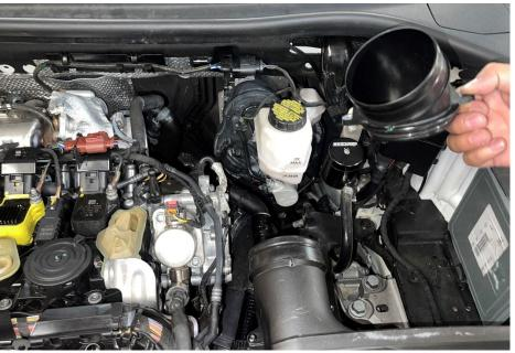
**Step 6**Install the 034 Turbo Inlet.
