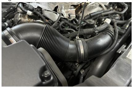
**Step 8**Remove the airbox/intake assembly from the car.
