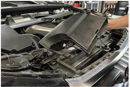
**Step 6**Remove the engine cover.
