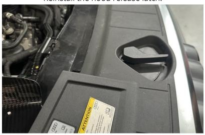
**Step 27**Reinstall the engine cover.
