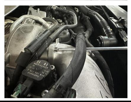
**Step 18**Attach the harness clips to the 034 turbo inlet.
