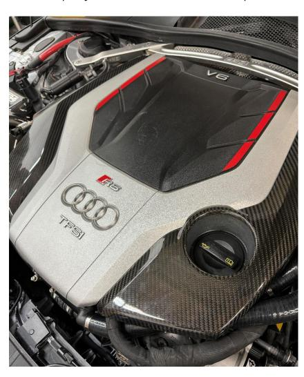
**Step 2**Remove the factory oil cap.
