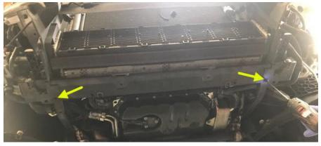
**Step 5** Using a 16mm socket, remove the 6 bolts (3 each side) securing the bumper crash bar brackets to the body.
