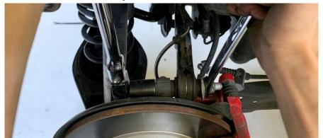
CONTROL ARM PAIR, DENSITY LINE, REAR UPPER ADJUSTABLE, 8J/8P/8V AUDI & MK5/MK6/MK7 VOLKSWAGEN
