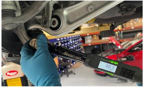
**Step 21** Using a 10mm socket, install the ride height sensor into the "front" lower control arm.
