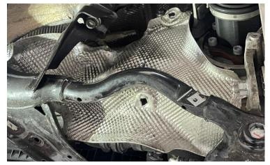
**Step 29** Using a combination of T30, T25, and a 13mm socket, reinstall the hardware for the underbody trays removed earlier.
