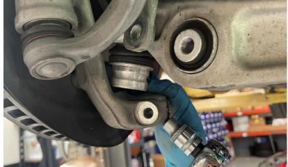
**Step 18** Using a 21mm wrench, install the loose ball joint into the "front" lower control arm. Torque to **140Nm.**
