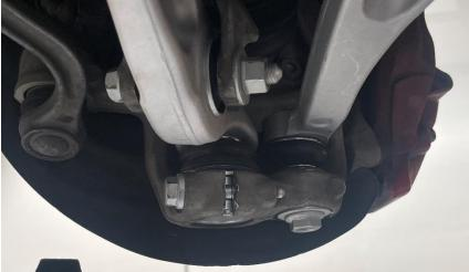
**Step 25** Using a 21mm socket, tighten the nut to the "rear" ball joint. Torque to **140Nm.**
