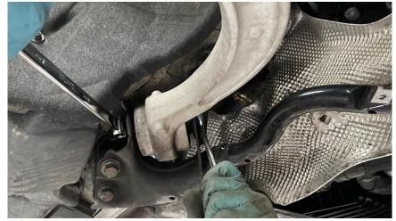
**Step 8** Using a ball joint removal tool, carefully break the rear ball joint free.
