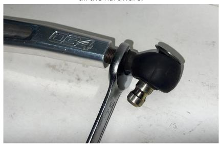
**Step 6**Slide the pin into the spherical joint.
