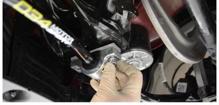
Step 10 Attach the sway bar end links to the 034 Rear Sway Bar using the factory hardware, but do not tighten fully. **Compress** suspension to static ride height. Torque end link hardware to 40 Nm + 180°.
