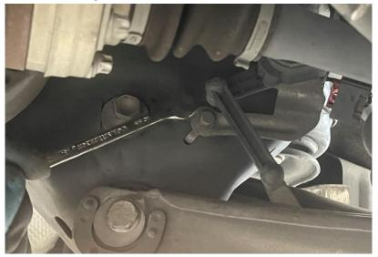
**Step 12**Unplug the connector to the ride height sensor.
