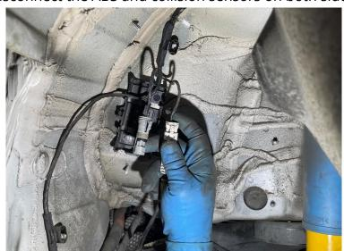
**Step 22**Remove the harness clips from the subframe.
