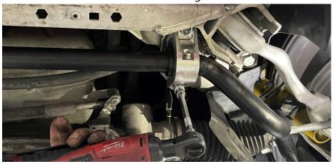
**Step 11**Torque the sway bar bracket hardware to **21Nm.**
