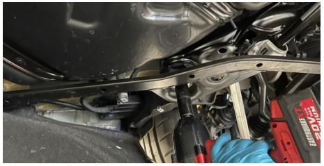
**Step 7** Using a 10mm triple-square, remove the hardware from the rear sway bar brackets.
