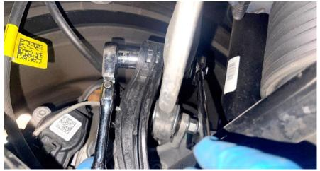
**Step 4** Using a 16mm socket and wrench, remove the lower end link hardware.
