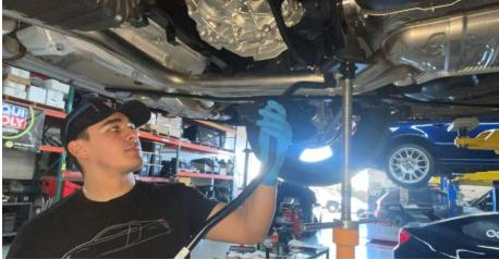
**Step 9** Apply grease to the rear sway bar bushings.
