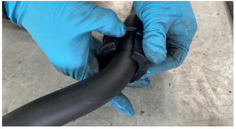
**Step 11** Snake the 034 rear sway bar into position. Hang the bar on the lower endlink hardware.
