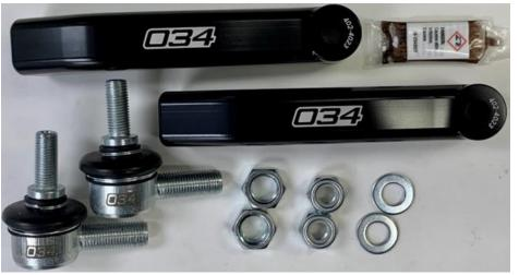
**Step 2**Apply half packet of anti-seize to each ball joint.
