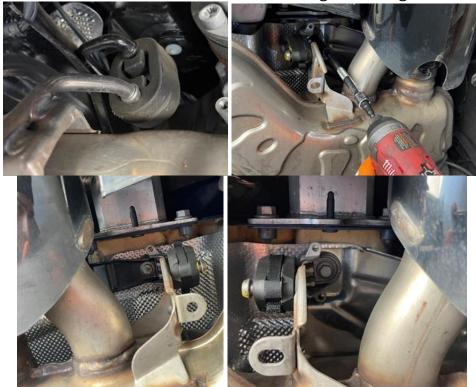
**Step 23**Reconnect the exhaust valve plug ends.
