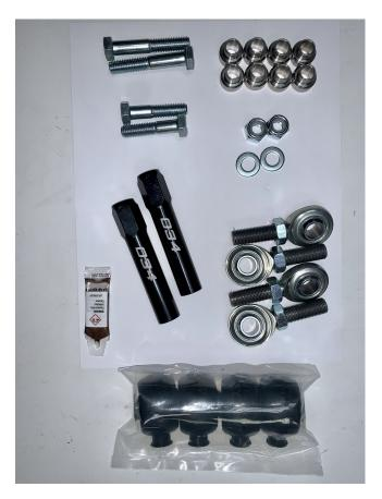
• Open anti-seize packets and apply to the end of heim joints, 1 packet should cover 2 joints.
