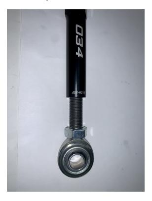
Use the length of the stock component as a starting point for the length of the 034 adjustable end links; expand or compress as best fits your needs
