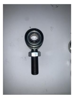
• The right-hand thread heim joints will thread into the hexagonal end of the billet end link
