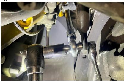
**Step 11** Torque all the nuts to **42Nm.**
