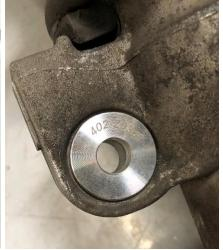
**Step 8**Install the 034 end link into the factory location.
