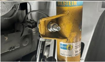
**Step 11**Torque all of the nuts to **42Nm.**
