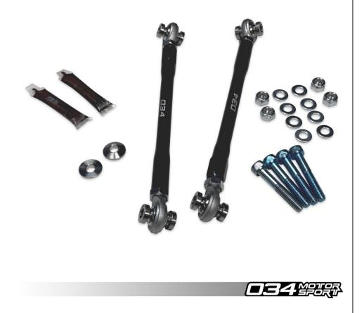
Designed to improve handling, road feel, and steering response, 034Motorsport's Motorsport Billet Adjustable Front Sway Bar End Links allow for instant transfer of suspension movement to the sway bar. These end links are also length adjustable to eliminate preload on the sway bar.
