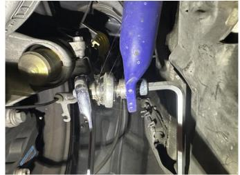
**Step 7** Using an 8mm Allen and a 17mm wrench, secure the end links to the strut housing.
