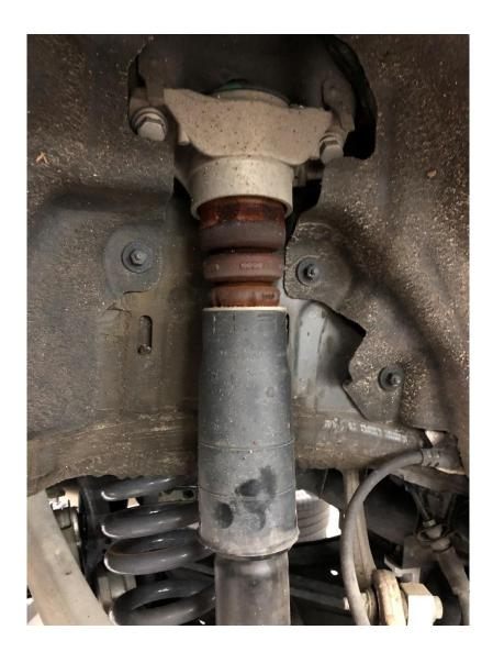
• Pull down on the rear bump stop to release it from the strut mount.
