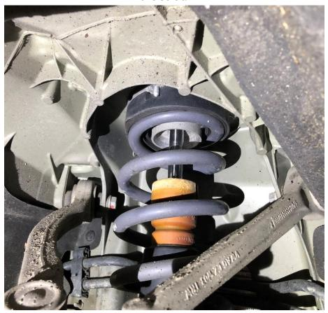
Pull down on the front bump stop to release it from the strut mount.
