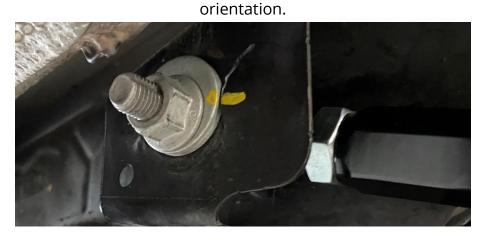
**Step 8**Thread the outter bolt back into the spindle.
