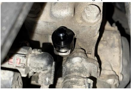
**Step 9**Install the silicone hose over the adapter nipple.
