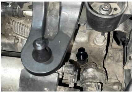
**Step 7**Install the transmission adapter shell over the adapter.
