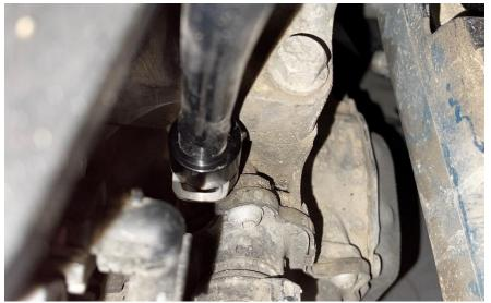
**Step 10** Using a 7mm socket, tighten one of the hose clamps to secure the hose to the adapter.
