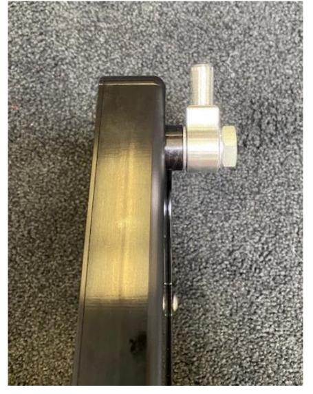
Tighten the banjo bolt to 20 NM, with the fitting outlet in this orientation.
