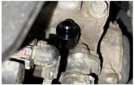
**Step 8** Install the adapter shell locking clip.
