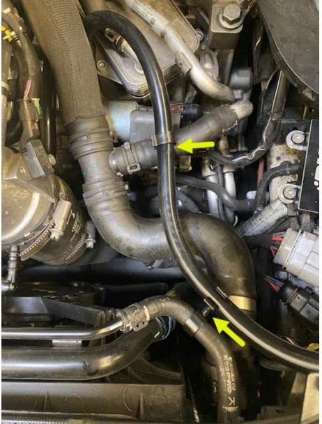
**Step 15** Using a T-30 Torx, remove these two headlight/radiator
