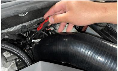
**Step 3** Pull the airbox off the mounting grommets.
