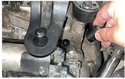
**Step 6** Install the 034 transmission adapter into the vent tube.
