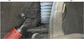
**Step 8**Unclip the ride height sensor harness.
