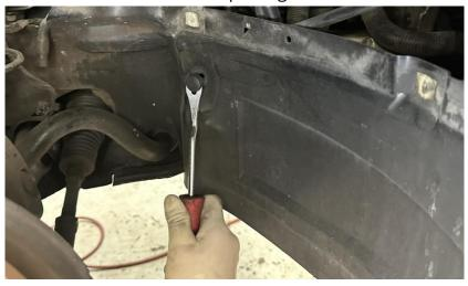
**Step 13** Unhook the hose and remove the lower splash guard.
