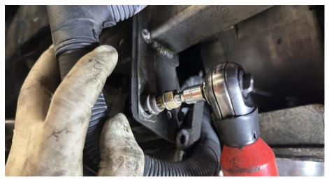
**Step 48**Reconnect the coolant pump.
