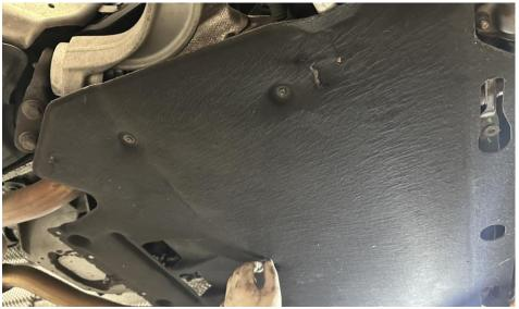
**Step 15**Using a T30, remove the side heat shields, near axles.
