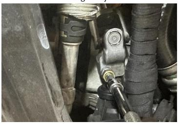
**Step 23** Disengage the steering column from the rack.
