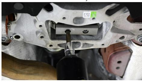
**Step 3**Remove the factory transmission mount bracket.
