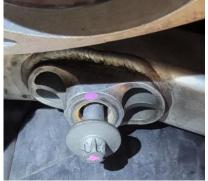
Using a 16mm socket, remove the top nuts of both engine mounts.
