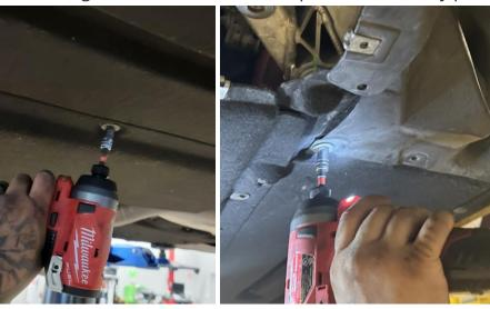
• Using an 8mm socket, remove the plastic side covers.
