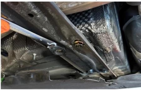
**Step 5**Remove the factory chassis brace.
