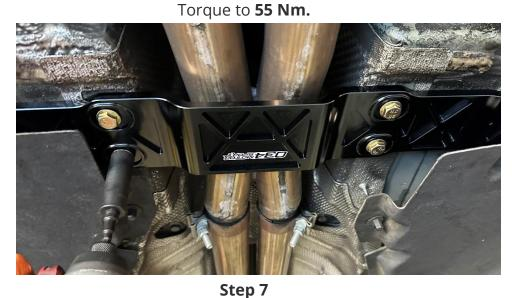
Using a 10mm socket, reinstall the bellypan hardware.
