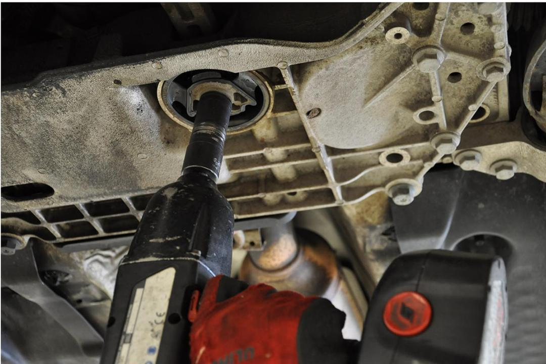
**Step 3** – With the factory bolt removed, you can install the Billet Aluminum Dogbone Mount Insert into the voids. It should be positioned with the 034Motorsport logo towards the front of the car.
