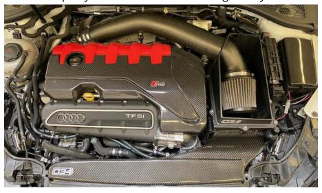
**Step 2**Unclip the factor "catch can" from the airbox.
