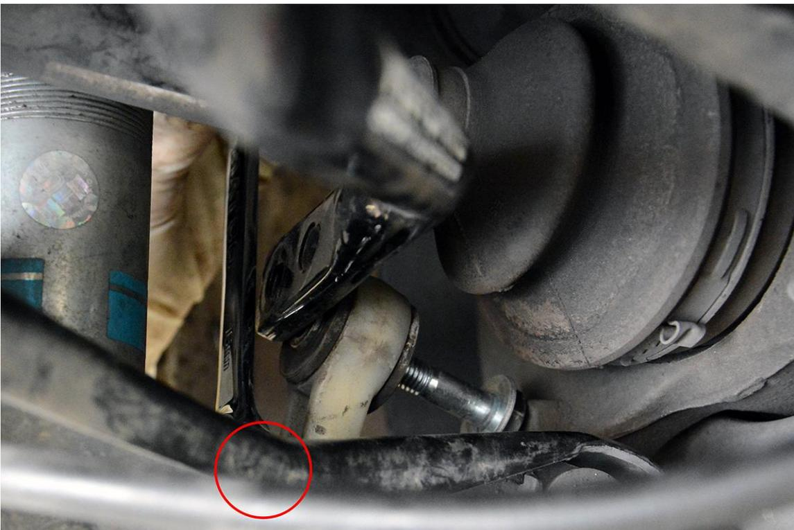
**Step 3** – This step will require some patience, and small hands help as well. If you have a patient friend with small hands, give him a call and invite him over to help. With a spacer installed on each side, secure the bottom of the Spherical Sway Bar End Link to the lower control arm with the supplied M10x50 Bolt and M10 Washer. Torque to 55 Nm.
