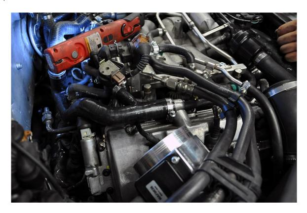
**Step 14** – Connect the hose from the billet check valve to the intake manifold. This may require you to rotate the hose on the clamp slightly. Tighten both clamps.
