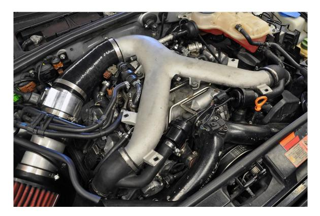
**Step 2** – Remove the PRV. Try not to break the clip, which is clearly an elaborate German test of intellect.
