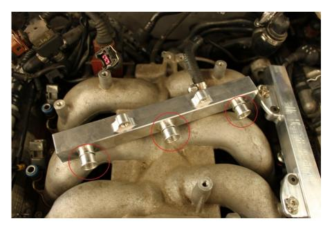
10. Install 034EFI Billet Fuel Rails using the provided brackets and hardware, taking care to align injectors into appropriate holes in manifold. Ensure that injector o-rings and/or injector hat o-rings are not externally visible; if they are, make sure you have the appropriate fuel rail bracket and spacing for your manifold and fuel injector choice.
