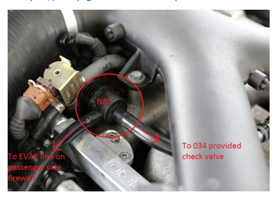
19. The other end of the line with two small  $\frac{1}{4}$ " nipples is for your diverter valves; run both diverter lines to this.
