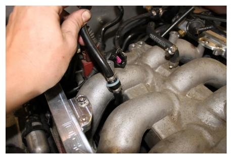
18. You may then run the line under the intake manifold or above it, with the check valve section going to the passenger side of the manifold, attaching to the N80 purge valve like pictured. The check valve will ensure you do not pressurize your EVAP system. If you have removed your EVAP system, you can plug/remove this section entirely.
