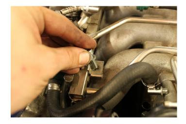
4. Remove injectors from factory fuel rail if installing new injectors; make sure that no o-rings fall off, or are left in the intake manifold or factory fuel rail
