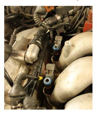
5. Remove N249 and N80 valves from the fuel rail; the 034EFI Billet Fuel Rail kit deletes the unnecessary N249. You can have this coded out via your software, you can leave the connector plugged into the valve. You may also want to cap off the vacuum pump check valve that is no longer utilized with the removal of the N249.
