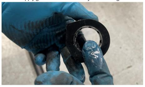
**Step 10**Separate the bushings along the split and wrap them around the sway bar.
