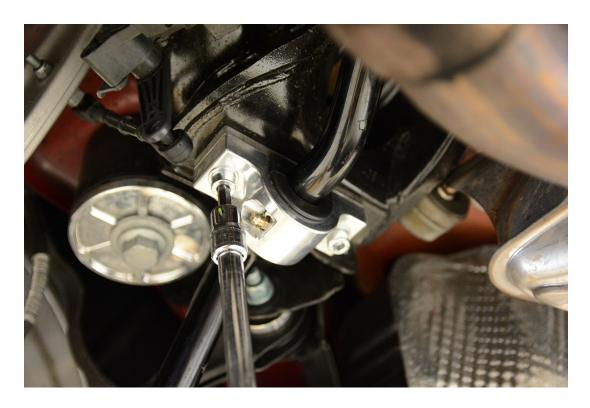
**Step 10** – Raise the exhaust and reinstall the exhaust hanger bolts you removed in Step 1.
