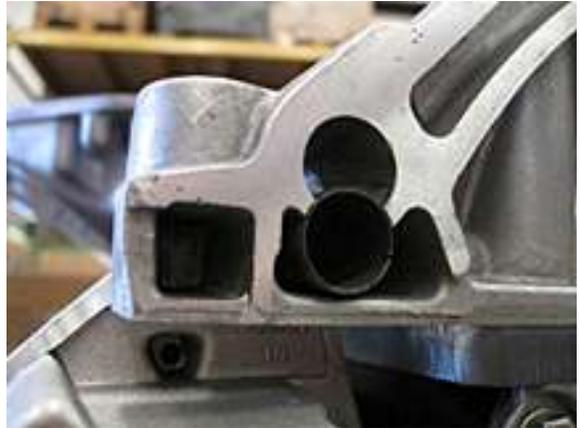
On V6 models the starter locating bushing must be relocated up by the thickness of the girdle:
