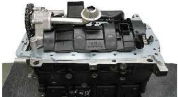
13.) The two girdle nuts located at the rear of the engine may interfere with the oil pan. Two grooves are required for proper clearance, but because the oil pan wall is narrow, an aluminum reinforcement block must be TIG welded to the opposite side prior to machining the grooves. Be sure there is enough space to thread in the oil pan bolts.
