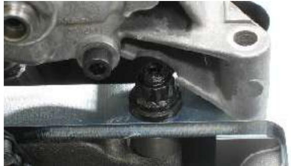
12.) Install the oil baffle.
