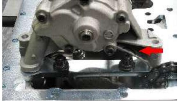
11.) Once there is appropriate tolerance, reinstall the oil pump and chain to factory specifications.
