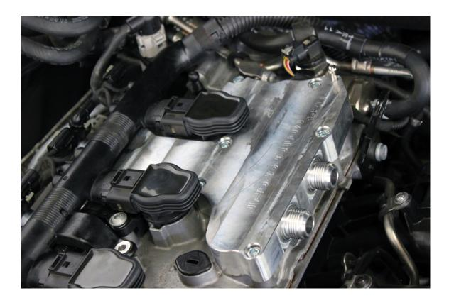
**Step 9** – Plug the coil harness back into all four coils, and secure the loom using the factory T30 Torx screw.
