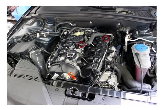
**Step 3** – Install the B7 Audi A4 2.0T FSI Intake Manifold Plug to black off the port where the valve cover breather to intake manifold hose was. Rotate the locking tab down to secure the plug against the plastic rib on the intake manifold plenum. If you intend to use this as a boost tap, unscrew the 1/8" NPT Plug, and replace it with a 1/8" NPT to appropriate barbed brass fitting for use with your boost gauge's vacuum line.
