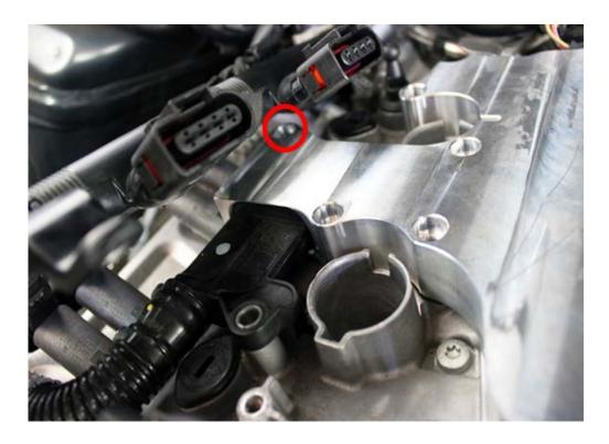
**Step 8** – Secure the Valve Cover Breather Adapter to the valve cover using the supplied M6x25 Bolts. The M6X22 Bolt goes into the left-most hole circled above. Secure the PCV assembly to compressor inlet tube to the valve cover using the factory T27 Torx screw.
