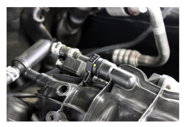
**Step 4** – Unbolt the T30 Torx screw securing the coil harness loom, and unplug the coil harness from all 4 coils. You can now access the single T25 Torx screw securing the PCV assembly to compressor inlet tube to the valve cover. Remove the T25 Torx screw and pull to remove the tube from the PCV assembly.
