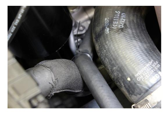
**Step 11** – Route the -10 AN Breather Hoses as pictured below, and secure to the Valve Cover Breather Adapter and Catch Can. Install the hose separator over the hoses and secure using the Allen bolt as pictured.
